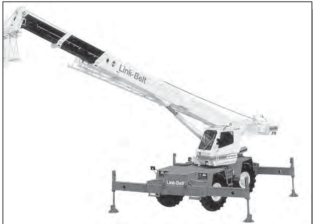
Figure 3.5-5 All Terrain Crane with Luffing
