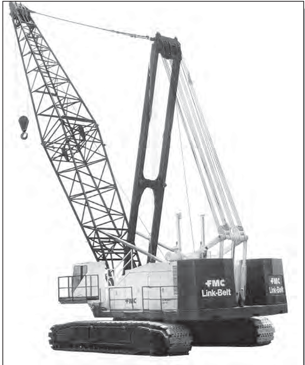
Figure 3.5-10 Lattice Boom Crawler Crane
