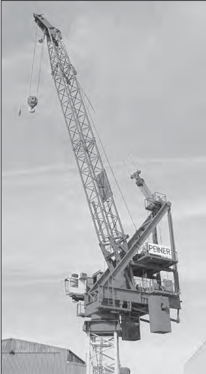
Figure 3.4-2 Luffing Jib Tower Crane
